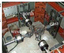
Figure 1: Biaxial test bench for flat cruciform specimens
