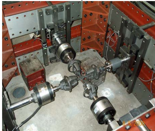
Figure 3 Bi-axial test set-up for tension-tension tests (VUB)
