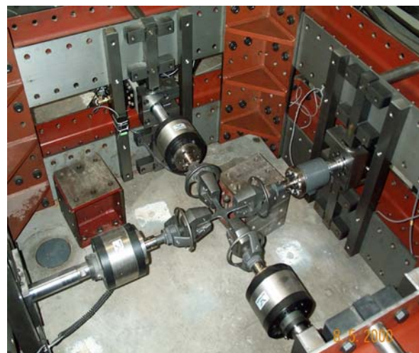
Figure 2: Biaxial test bench for cruciform specimens loaded in tension/tension.
