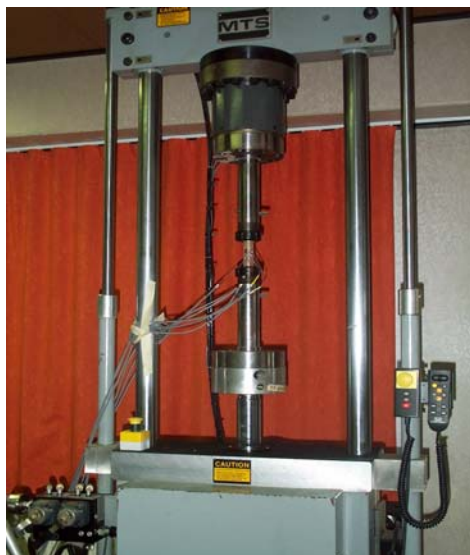
Figure 1: Biaxial test bench for specimens loaded in tension/compression combined with torsion.
